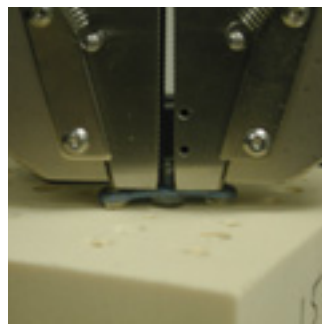
Figure 2: Pullout test depicting a UNIPLATE Anterior Cervical System as it is extracted from 15pcf sawbone.
